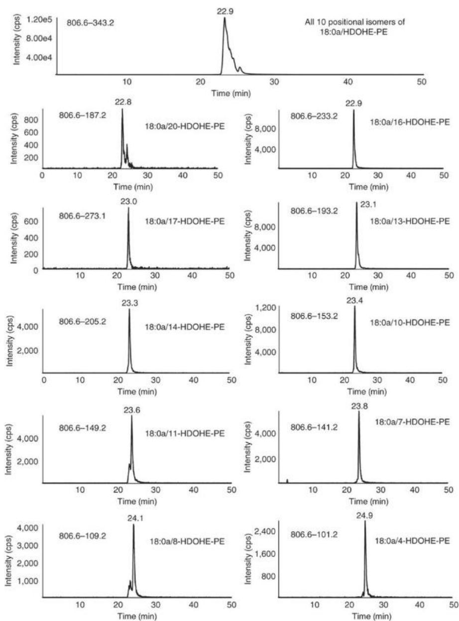
All isomers have  $m/z$  806.6. HDOHE-PE lipids were generated by air oxidation, as described in Step 1B, and purified by reverse-phase HPLC. A sample was separated using LC/MS/MS as described in Steps 12–14. Elution was monitored by either  $m/z$  806  $\rightarrow$  343 (all positional isomers) or product ions specific for each positional isomer.
