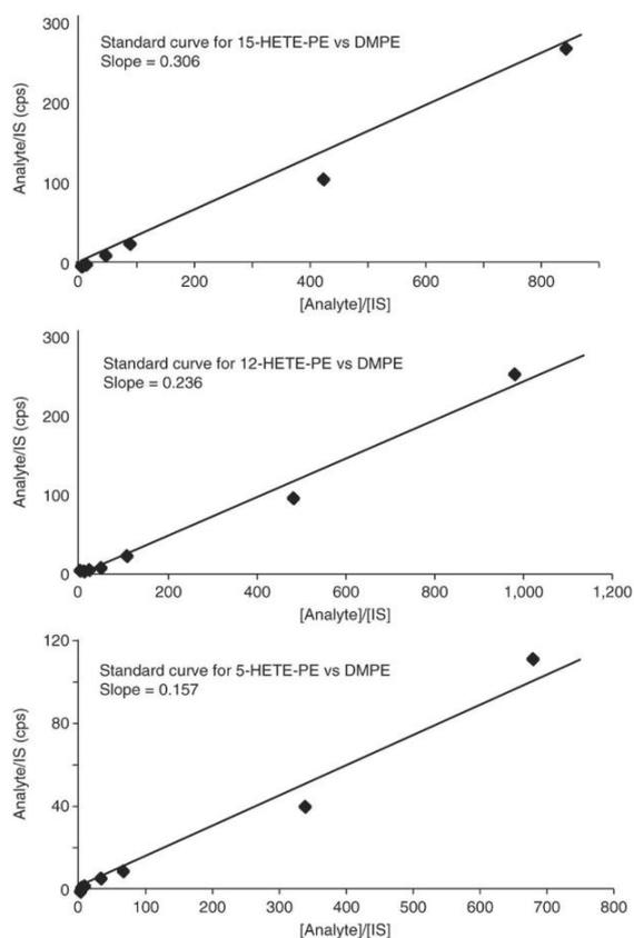
Standard curves were created by adding a fixed amount of DMPE to varying amounts of the standard HETE-PE positional isomer mixture, generated by air oxidation, and analysed using LC/MS/MS as described in Steps 12–14.
