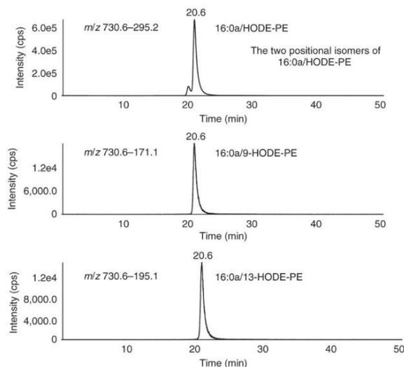
Isomers have m/z 730.6. HODE-PE lipids were generated by air oxidation, as described in Step 1B, and purified by reverse-phase HPLC. A sample was separated using LC/MS/MS as described in Steps 12–14. Elution was monitored by either m/z 730 → 295 (all positional isomers) or product ions specific for each positional isomer.
