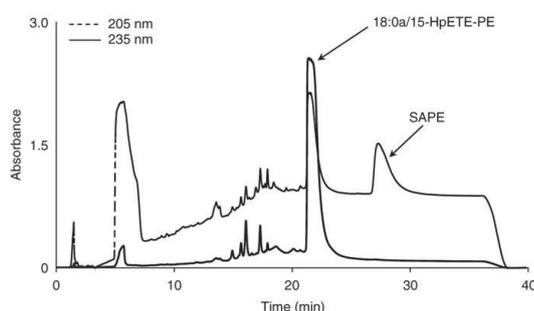
SAPE was oxidized using soybean LOX as described, then lipids were extracted and 18:0a/15-HpETE-PE was purified using reverse-phase HPLC, with monitoring at 235 nm (product) and 205 nm (substrate). The esterified eicosanoid elutes at about 21–22 min.
